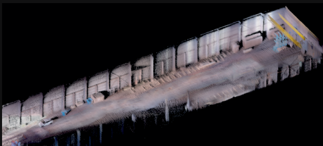
Total View: 3D Map in GNSS-denied Environment, colored by Camera RGB Values
